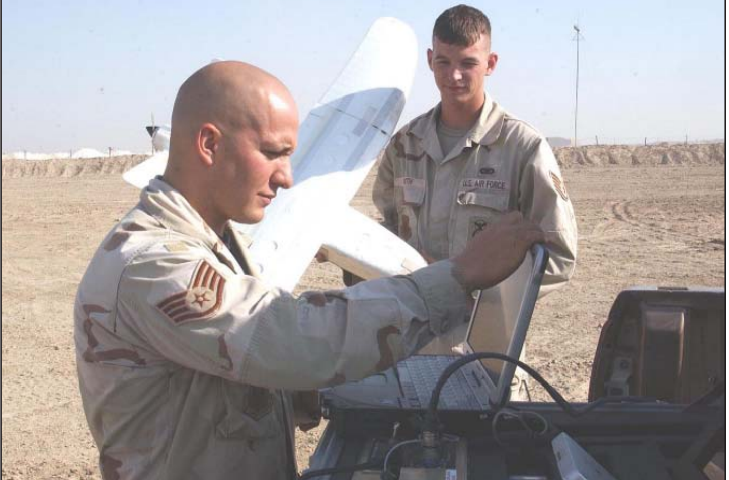
▲ READY FOR TAKEOFF: Staff Sgt. Joseph Vialpando (left) and Staff Sgt. Michael Roth prepare the 'Desert Hawk' aircraft for flight. The lightweight aircraft is part of the Force Protection Airborne Surveillance System used at Tallil Air Base to see over the horizon looking for terrorist activities.
