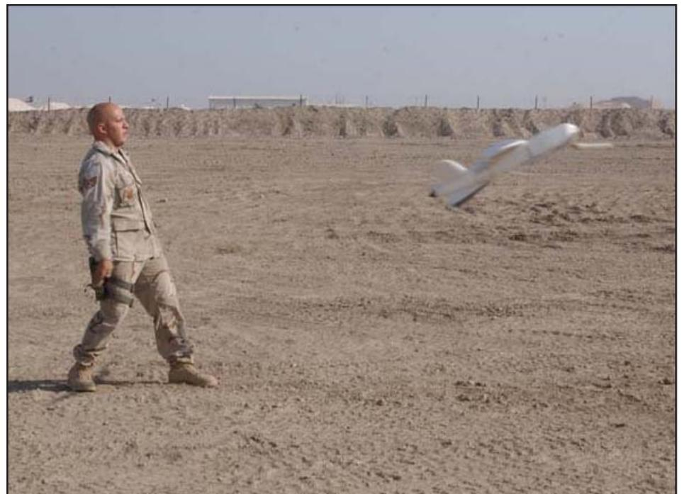
▲ **UP AND AWAY:** Staff Sgt. Joseph Vialpando recoils back after releasing the Desert Hawk aircraft. The four-foot long plane relies upon a bungee cord catapult system to provide acceleration for takeoff.
