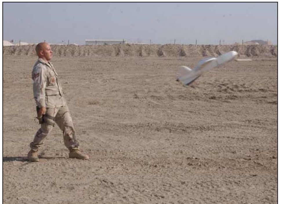
▲ UP AND AWAY: Staff Sgt. Joseph Vialpando recoils back after releasing the Desert Hawk aircraft. The four-foot long plane relies upon a bungee cord catapult system to provide acceleration for takeoff.
