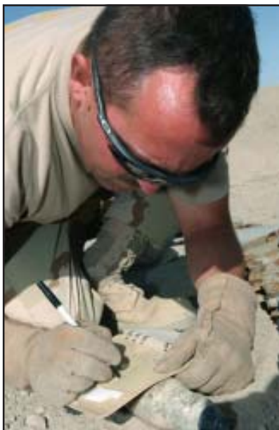
▲ TAKIN’ NOTES: Tech. Sgt. Tom Cowern, 332nd ECES EOD Flight craftsman, documents an Iraqi M73, a 60 millimeter, high explosive filled, mortar, with an Italian PDB 335 Fuze prior to detonation.
